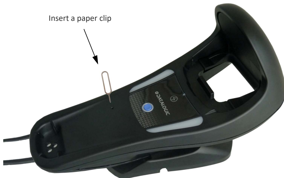
Figure 13 - Disconnecting the cable
